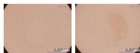
[Fig 4] Adhesive failure (left) vs mixed failure (right).
